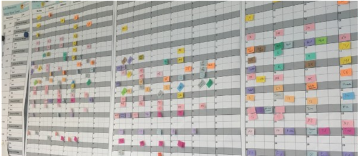
Figure 2: Example of a pull planning sequence developed in a last planner meeting using post-it notes [7].
